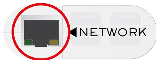
The easiest way to connect the Gateway to the internet is to plug an Ethernet cable into the port on the end of the device.
