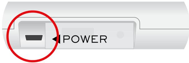
Connect the power supply to the Gateway. The red power light will come on solid for about 30 seconds as the unit is booting up. It will then begin flashing to indicate the Gateway is in Discovery Mode.
