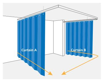
Curtain A: 4.5m length for short sections dividing cubicles Curtain B: 7.5m length for long sections i.e. curved track at front of cubicle (2.5m length also available for small cubicles, privacy curtains, across windows - fits sizes 0.5m to 1.8m width areas)
