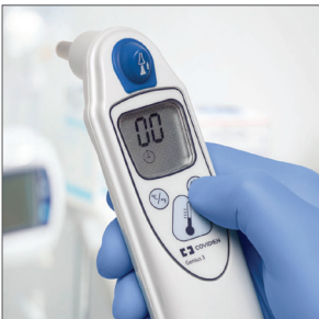
To change the temperature display, press and hold the C°/F° button for 2 seconds when the LCD screen is active.
