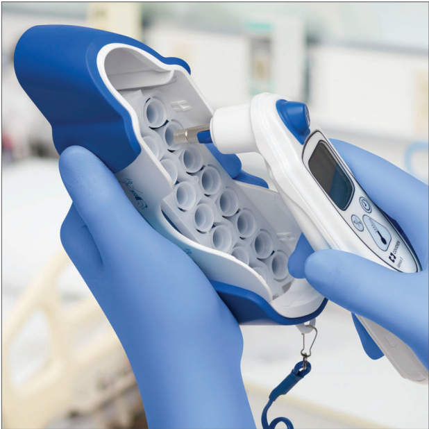
Attach a probe cover by aligning the silver tip with a probe cover and push straight down until you hear a snap. Inspect the membrane on the end of the probe cover. If a hole or tear is visible, discard and attach a new probe cover.
