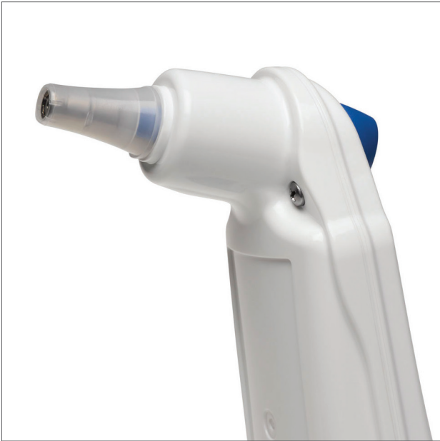
Ensure the probe cover is securely seated on the probe. The silver probe should not be showing. A probe cover MUST be used.
