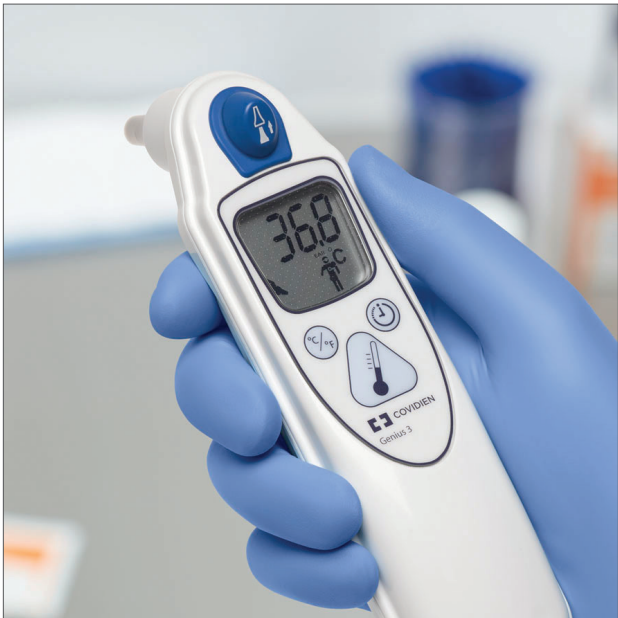
To recall the last temperature, press and release the scan button before loading another probe cover. Loading a new probe cover will erase the last temperature taken from the memory.
