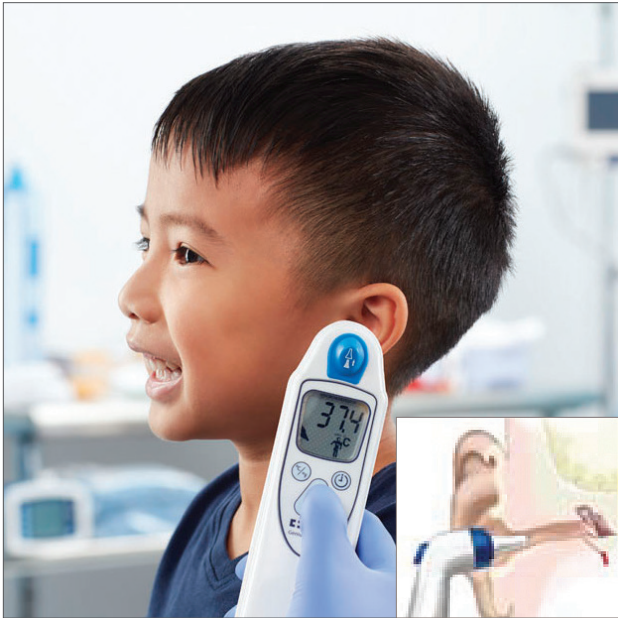
Insert the tapered probe tip. Align the probe at the entrance of the patient's ear canal. Immediately press the large triangular scan button located in the center of the handle. A triple beep will sound when the scan is completed.
