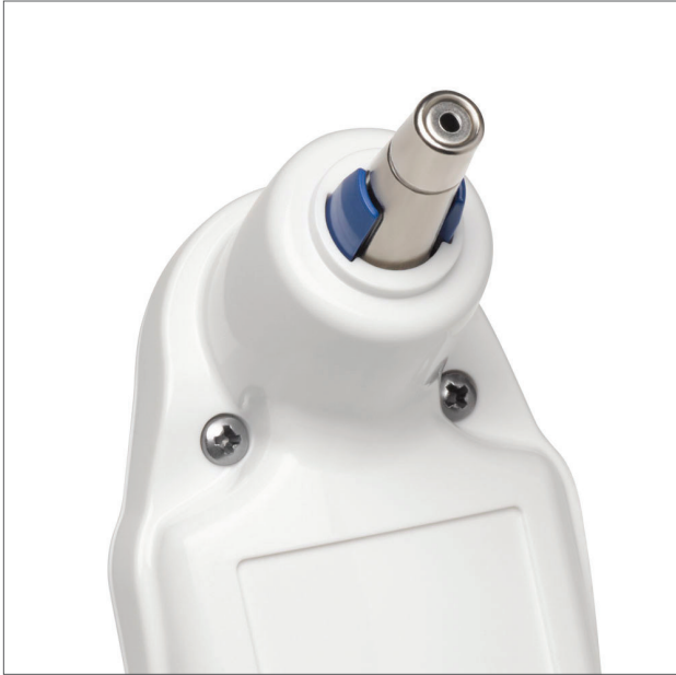
Inspect the probe lens. It should be shiny and free of cracks or debris without a probe cover attached. (Clean lens with a dry lint-free swab or lens wipe if needed.)
