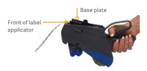
Turn the label applicator over and squeeze the handles (A+B) repeatedly to tighten, self align and cause a printed label to be dispensed.
