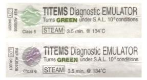
**Wet:** Emulator laminate will "bubble" when excessive moisture has been present in the sterilizing process.
