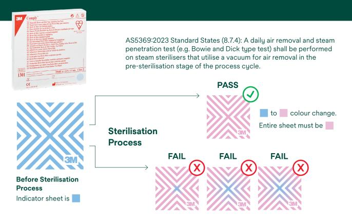
Any evidence of blue colour on the indicator sheet means Bowie Dick Test Failure
